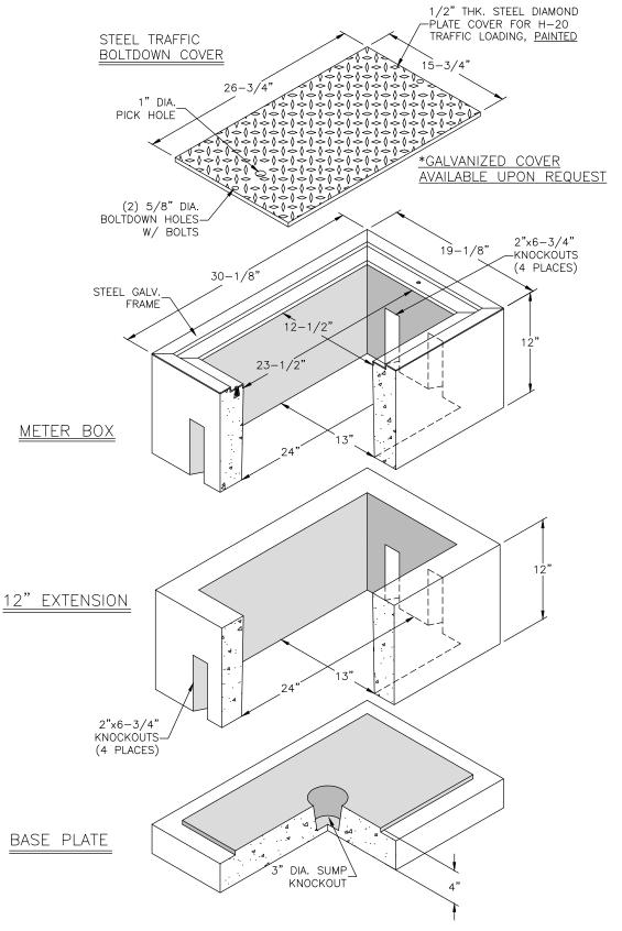
No. W5-T Series Meter Box W/ H-20 Wheel Loading Cover Per CALTRANS Specifications
