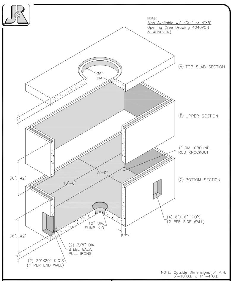
5'-0" X 10'-6" CLOSED BOTTOM **ELECTRICAL MANHOLE VAULT** (SPECIAL DESIGN AVAILABLE)
